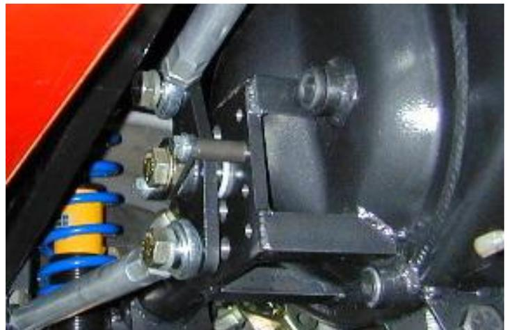
**WARNING:** When tightening center bolt be sure that bell crank has resistance to hand motion but is not locked up. Production tolerances may require you to sand either the ends of the sleeve or the shoulders of the bushings to fit snugly when lubricated and torqued. If it is loose it will wear out prematurely and may rattle. If it is too tight bind may occur affecting performance and in extreme cases damage may result.
