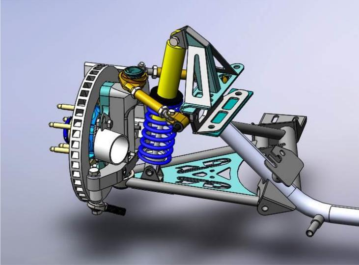
After removing K member, spindles, struts, etc., and thoroughly cleaning subframe areas for installation of SLA kit, brake lines and brackets mounted to the outside of the subframes above the K member will have to be relocated to suit the individual need of the vehicle and brake system employed. It is best to perform this function during final assembly after GR40 SLA is fully installed. **It is recommended that custom tailoring of brake lines be done by a professional.**
