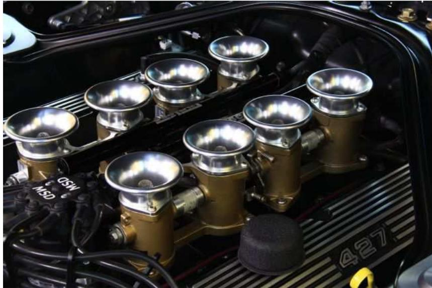
**On top is an Inglese induction eight-stack system with FAST EZ-EFI fuel injection.**
