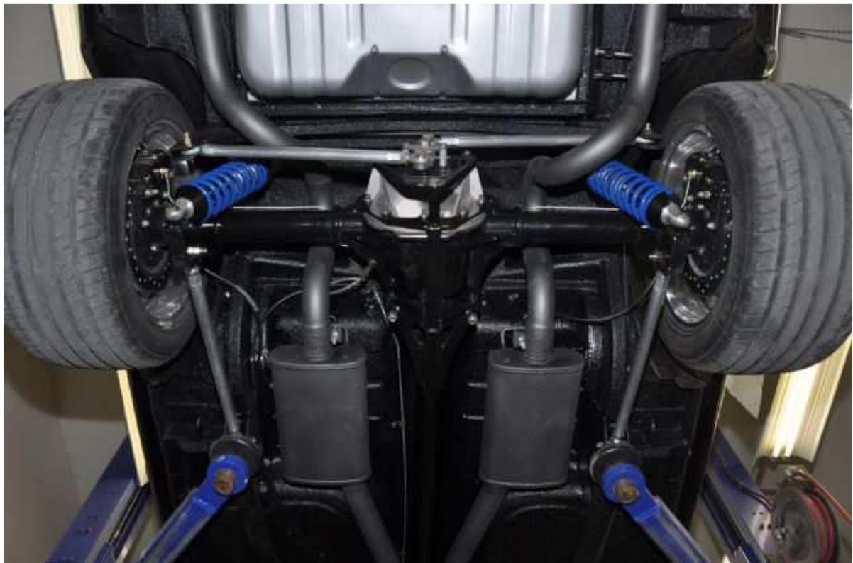
**This isn't your garden-variety classic Mustang restomod. Alec and Eddy, along with the spirited attitude of Scott Brideau, created a one-of-a-kind 1967 fastback with Griggs underpinnings, power rack-and-pinion steering, Wilwood disc brakes, MagnaFlow mufflers with 2 1/2-inch pipes, and a Fox body 8.8-inch rear axle.**
